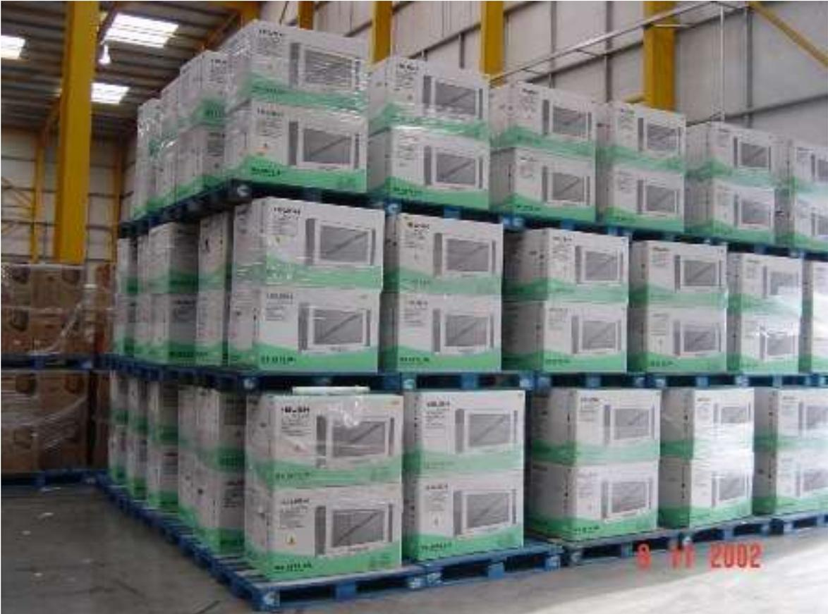
**Figure 8 – Block stack**
